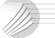
Cap Sheet – Polyester\* Clearcoat – Polyurethane Film – Polyurethane Adhesive - Acrylic PSA
