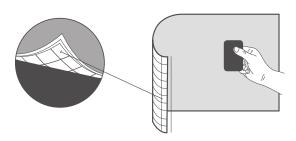
Figure 1: 3M<sup>™</sup> Comply<sup>™</sup> Air-Release Channels
